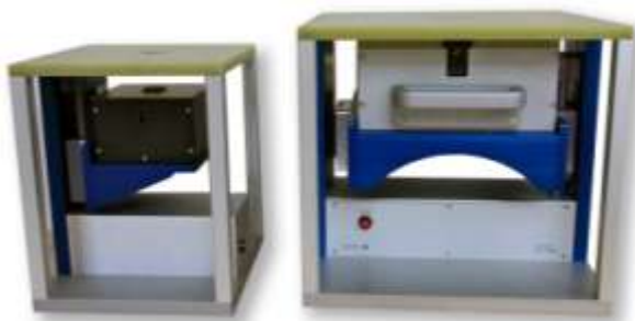
profile NMR-MOUSE models PM 5 and PM 25 mounted in high precision lifts.
